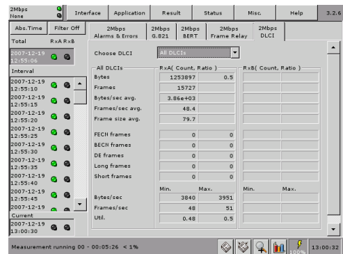
Fig. 33 The CMA 3000 monitors a large number of parameters for up to 50 DLCIs simultaneously.
