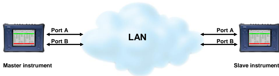
Fig. 11 RFC 2544 testing of asymmetrical Ethernet links using two CMA 3000s. Two links can be tested simultaneously
